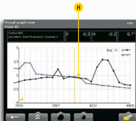
The result displayed as "Best fit around 0" (H), and with sharp graph.
